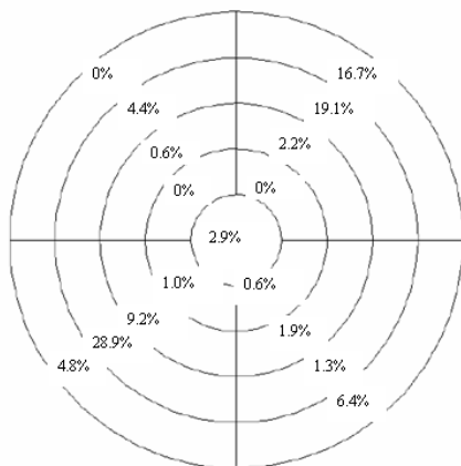
4.5% of the water volume collected within a radius of 20cm (fails EU standards).
