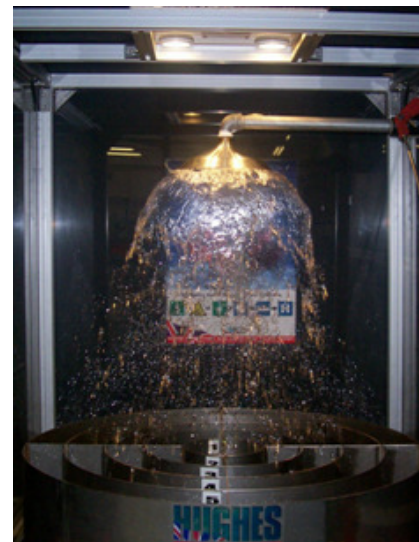
Figure 11: Modified filmer design (60 l/min)..
