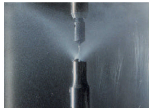
Ultrasonic Atomization of Low Melting Point Alloy and (top left) Gas Atomizer Close Coupled Nozzle
