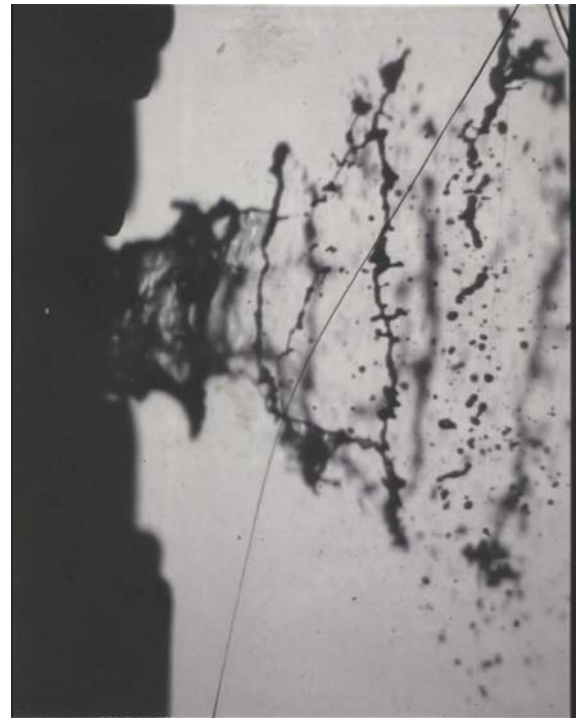
Advanced optical methods analyse break up into 50 micron drops near insert
